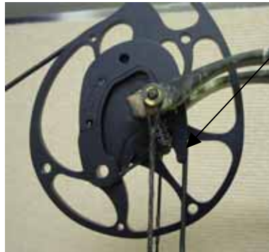
Cable makes contact with the flat on the module on the upper cam.
